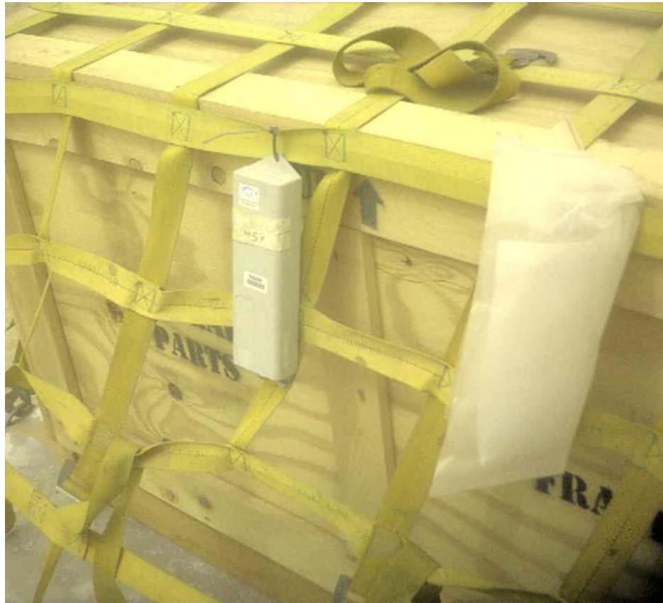
Figure 13.4: SAVI RFID Tag on a Pallet in Kuwait
