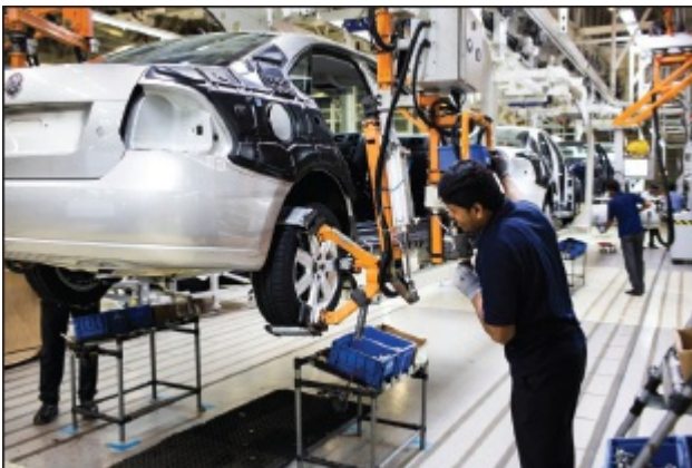
An employee uses a robotic arm to fit a wheel onto a Volkswagen AG Vento automobile on the production line at the Volkswagen India Pvt. plant in Chakan, Maharashtra, India.
