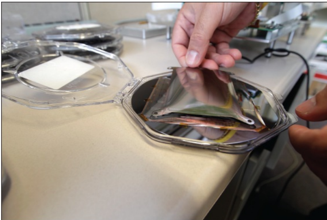
John Maltabes, research engineer at Hewlett-Packard, takes out a thin flexible electronic display that has etched resistors and uses self-aligned imprint lithography technology for testing at Hewlett-Packard Laboratories.
